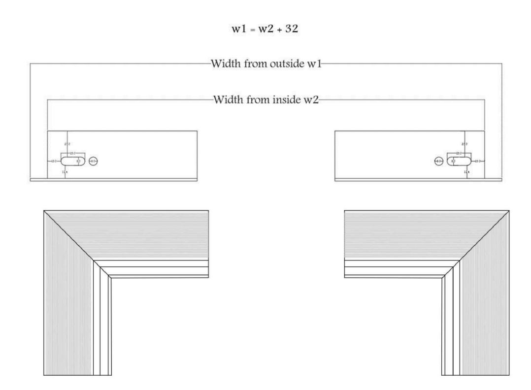
• Frame Dimensions – Interior and Exterior Sides
